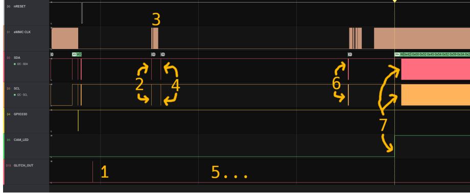
Fig. 2: Logic analyzer capture of the ARM9 boot ROM extraction process. Some time after reset release, a first fault is injected (1). The ARM7 payload then starts mimicking the regular boot ROM execution (2-4). After this, the SoC hangs as the ARM9 waits for the ROMs to be locked away (5), which the ARM7 payload does not do. After injecting a fault into the ARM9 successfully (not pictured on the GLITCH_OUT line), the console continues booting (6) and the result is transferred over I2C (7).
